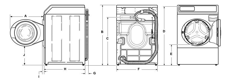
A 611 mm [24.06 in.] D 1006 mm [39.61 in.] G 52 mm [2.04 in.] J 333 mm [13.1 in.] B 1027 mm [40.42 in.] E 371 mm [14.6 in.] H 704 mm [27.73 in.] C 813 mm [32 in.] F 683 mm [26.875 in.] I (with door closed) 40 mm [1.59 in.]
